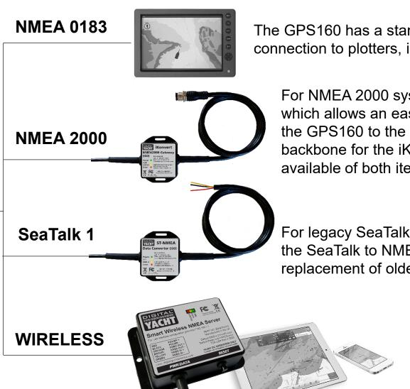
The GPS160 has a standard NMEA 0183 output for connection to plotters, instruments and systems
