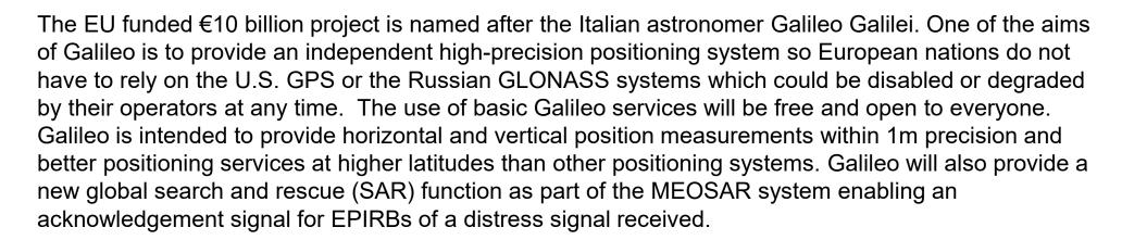
There are currently 22 satellites in usable condition (operational and contributing to the service provision), 2 satellites are in "testing" and 2 more are marked as not available. The final constellation should be deployed by 2020 and will consist of 30 satellites (24 operational and 6 spares).
