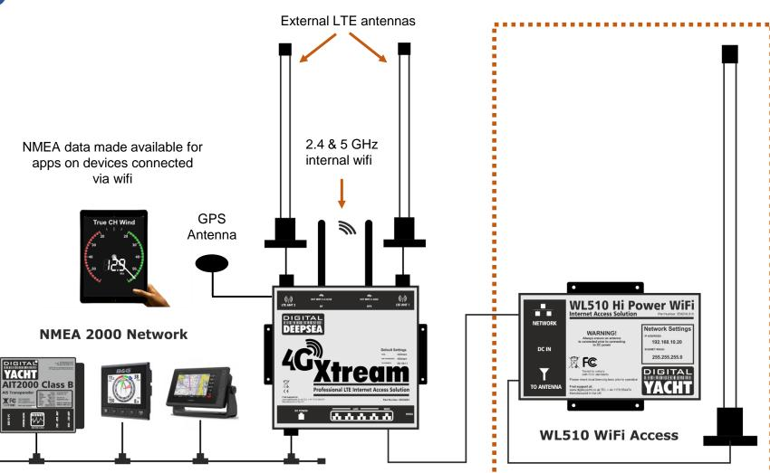
NMEA navigation and instrumentation data connected via built in interface to allow iPad and tablet app connectivity
