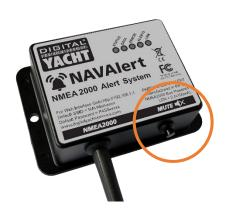
Alarms can be acknowledged/ silenced via the mute button fitted to the unit or via a compatible NMEA 2000 multi function display
